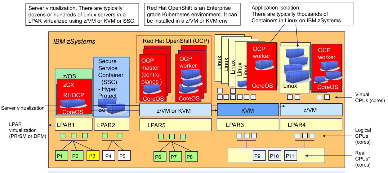
P1 – P11 are Central Processor Units (CPU -> core) or Integrated Facility for Linux (IFL) Processors (IFL -> core) or ZIIP cores in z/OS
