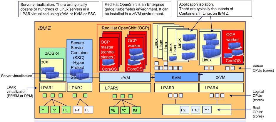
P1 – P11 are Central Processor Units (CPU -> core) or Integrated Facility for Linux (IFL) Processors (IFL -> core)
