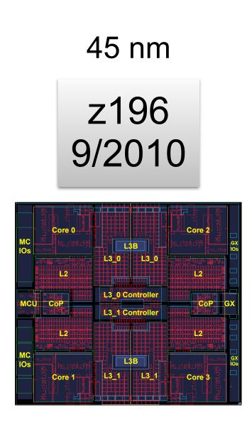
Top Tier Single Thread Performance, System Capacity **Accelerator Integration** Out of Order Execution Water Cooling PCIe I/O Fabric RAIM **Enhanced Energy Management**
